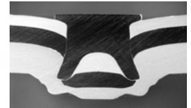
EN AW-5754, t = 1.0 mm DP1000, t = 1.5 mm Die-cast aluminium, t = 2.7 mm HDZ 5.5 x 7 SK H4 Almac
