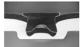
22MnB5, t = 1.2 mm Die-cast aluminium, t = 2.7 mm HDZ 5.5 x 5 SK H4 Almac
